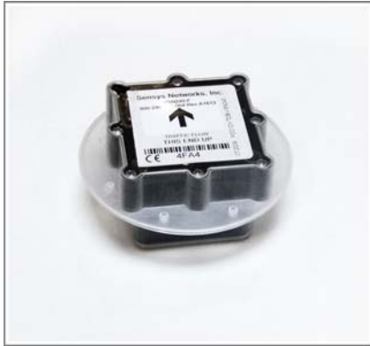
Figure 3.8 – Finished Sensor and Shell Assembly
